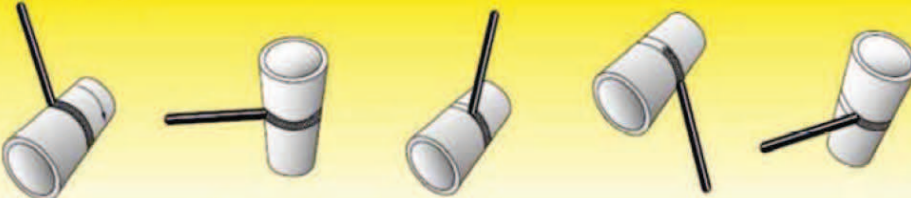
Pipe rotates horizontal axis Downhand: PA/1G Pipe fixed vertical axis, welding horizontal-vertical: PC/2G Pipe fixed horizontal axis, welding uphill: PH/5G Pipe fixed horizontal axis, welding downhill: PJ/5G Pipe fixed with axis under 45° welding uphill: H-LO45/6G
