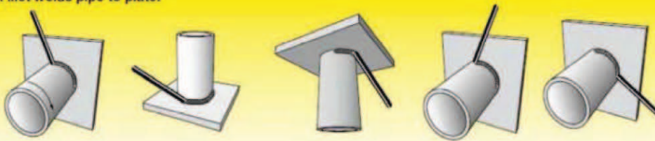
Pipe rotates horizontal axis Downhand: PB/2FR Pipe fixed vertical axis, welding horizontal-vertical: PB/2F Pipe fixed vertical axis, welding overhead: PD/4F Pipe fixed horizontal axis, welding uphill: PH/5F Pipe fixed horizontal axis, welding downhill: PJ/5F
